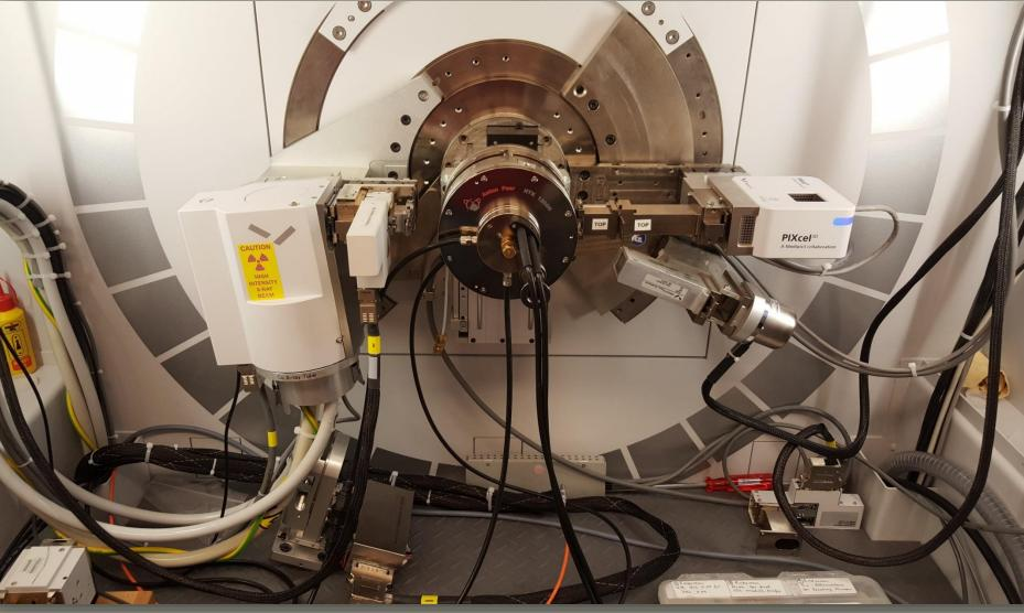
Panalytical Empyeran XRD machine with Anton Paar high temperature stage
