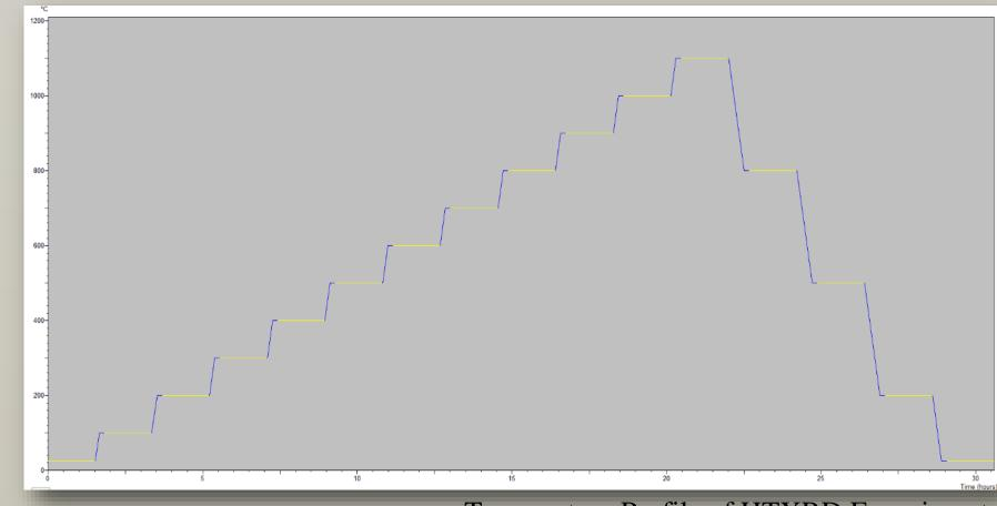
Temperature Profile of HTXRD Experiment
